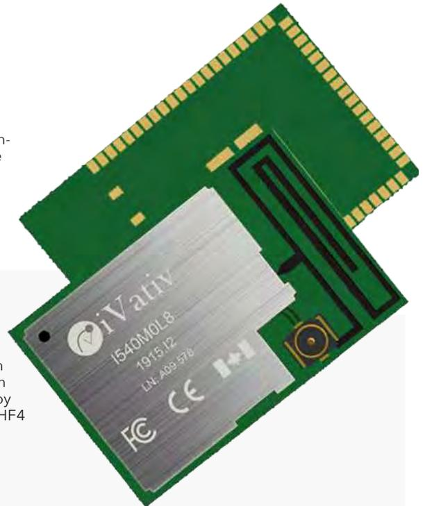
of >1000m, low power consumption and reliable radio operation, this tuned RF module contains—in addition to the antenna—the entire analogue front-end including crystals. Operating temperature range is -40 to 85°C without restrictions.
