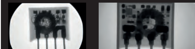
Fig 4 Decapsulation (L) DUT; (R) known good
